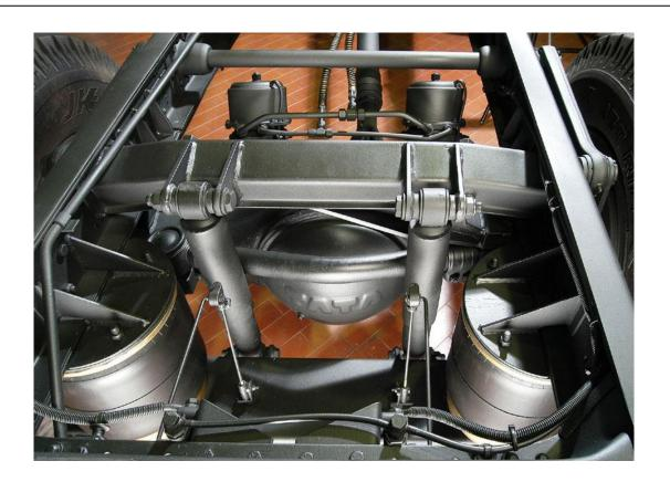
The conventional leaf springs (L.S.) in the Suspension System of a Vehicle has a load / deflection Curve which has a constant slope. But, with very low available travels and static deflections as also high hysterisis, there are obvious constraints with regard to achieving comfort levels inside the vehicle. In spite of shock absorbers used in "Tandem" the leaves of the bundled spring are subject to fatigue as well as impact stresses due to which vibrations and shock are routinely experienced.
